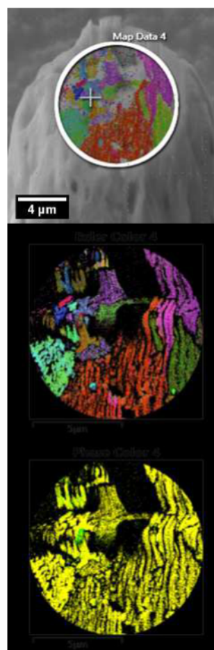
Figure 4. EBSD grain orientation (middle) and phase map (bottom) from the FIB cross-section (top) of the particle shown in Figure 3.
